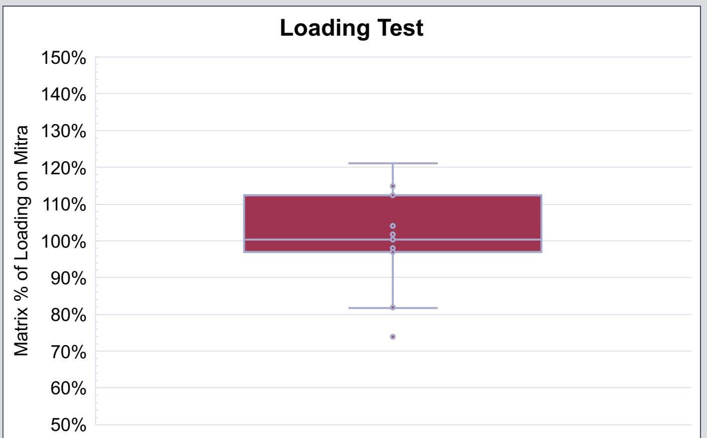
Figure 10. Mitra VAMS Loading Test: Mitra VAMS devices used for the microsampling stability test were weighed before and after sample loading. The experiment showed consistent reproducibility, with the majority of samples falling within ±20% of the nominal volume.
